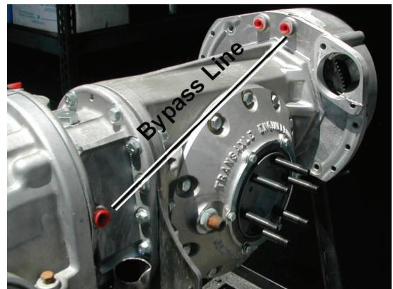
Repeat this procedure to eliminate any air pockets any time the oil lines are disconnected for service or repair. This will also help flush out any minor contamination in the oil system.
