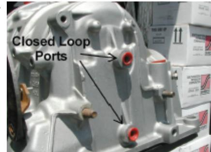
If an **oil temperature** gauge is installed (highly recommended) we recommend that you install the oil temperature sender in the return line where it exits the heat exchanger or oil cooler.
